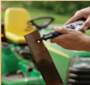
Sharpening a lawnmower blade
