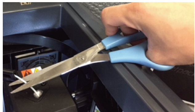
Figure 3: Cut filament before the intake.
