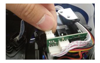
f. Re-attach the fillament run out switch connector from previous step. Fasten the two screws on the top of the extruder top cover using the 2.5 mm hex wrench. Fasten right screw on the bottom of the extruder removed in step b using the T10 Torx screwdriver. Inset filament into extruder, and resume normal printer usage.
