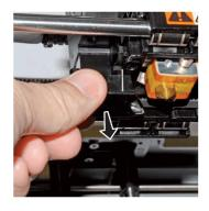
Step 7: Unscrew the turbo fan mounting bracket screw from the left back side of the extruder assembly.
