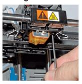
Step 17: Reconnect the fan wire connector. This connector is marked with black ink. (Red and black to red and black wires).
