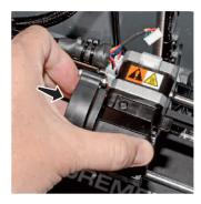
Step 22: Insert and tighten the back left screw for mounting the turbo fan bracket.
