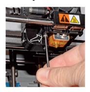
Step 6: Remove the fan baffle from the turbo fan.
