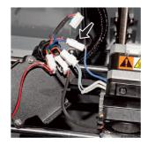
Step 20: With all wires connected, neatly place the connectors into the open area of the turbo fan bracket. Make sure wires lay flat underneath the stepper motor.
