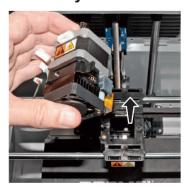
Step 15: Replace the new extruder assembly onto the extruder carriage.
