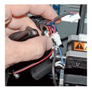
Step 21: Move the turbo fan bracket next to the extruder capturing the wire connectors between the bracket and the extruder assembly.
