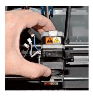
Step 16: Insert and tighten both screws, left and right, to secure extruder assembly to the extruder carriage.
