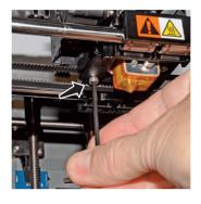
Step 23: Insert the fan baffle into the turbo fan.
