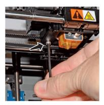
Step 8: Move the turbo fan bracket and turbo fan away from the extruder assembly. This will expose the wire connections.
