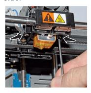
Step 14: Remove the extruder assembly.
