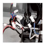
Step11: Disconnect the fan wire connector. This connector is marked with black ink. (Red and black to red and black wires).
