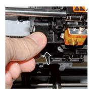
Step 24: Insert and tighten the fan baffle screw on the front left side of the extruder assembly.
