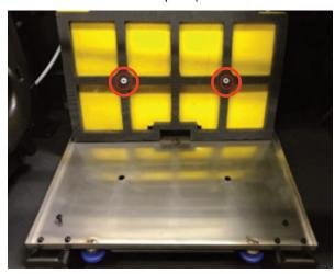
b. Raise the platform up and reinstall the 2mm Allen screws, with the small washers and nylock nuts. Refer to step 3.
