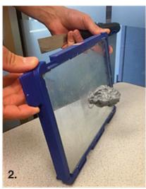
b. Ensure the build plate is well secure and will not slip once object removal tool is being used.
