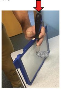
c. Repeat this process if needed until the part detaches from the build plate.
