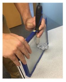
b. Give a firm bump on the top part of the object removal tool (see red arrow).
