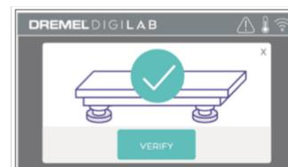
4. If the build platform is too low, adjust the knob by rotating left until you hear a “beep” and the touch screen indicates that it is ready to verify that the bed is level.
