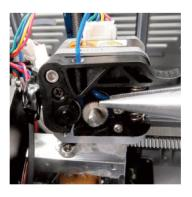
Step 8: Replace the stepper motor and fan. Tighten the 2 fan screws in place. Note: Screws should be hand tightened. Do not over tighten or you may damage the extruder fan.
