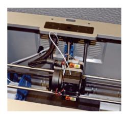
Step 2: Unload filament from the extruder.
