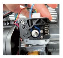
Step 7: Remove the clogged filament with a needle nose pliers. Note: Make sure to remove all remnants of the clogged filament and discard appropriately. Any remaining filament may cause the printer to not work properly.
