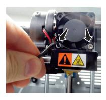
Step 6: Remove the fan exposing the drive gear.
