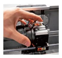
Step 5: Open the front door, then using the allen wrench, loosen the two screws on the front fan.
